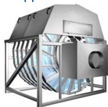
The tank version of Hydrotech Discfilter is provided with an internal emergency by-pass and a level weir to maintain the water level after the filter. The versions without tanks are designed for installation in a concrete channel or basin.
