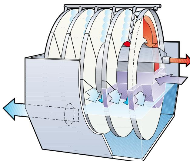
**Flexibility is a key word** for the Hydrotech Discfilter. The patented design of the panels means that replacement requires minimum service and downtime. If there is a change in operating or performance needs, the design also accommodates an easy switch to a filter media with a different size of opening.
